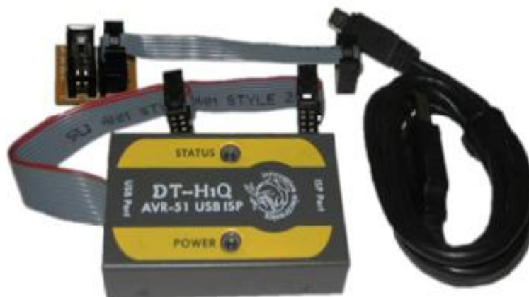
Gambar 3.10. Downloader DT-HiQ AVR-51 USB ISP. (Sumber : Datasheet . Downloader DT-HiQ AVR-51 USB ISP : 1-5)
