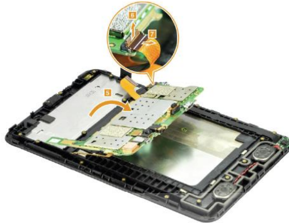
Gambar 4.48. Melepaskan System Board
