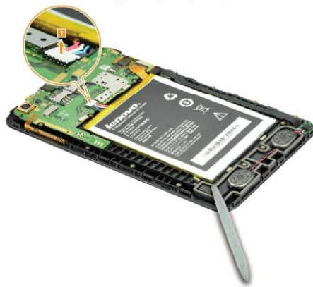
Gambar 4.45. Membuka Battery Pack
