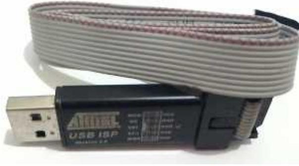
**Gambar 3.7** Downloader ATMEL USB ISP (USBasp)
