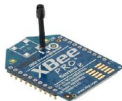
**Gambar 2.7** Xbee Series 2 Wire Antenna
