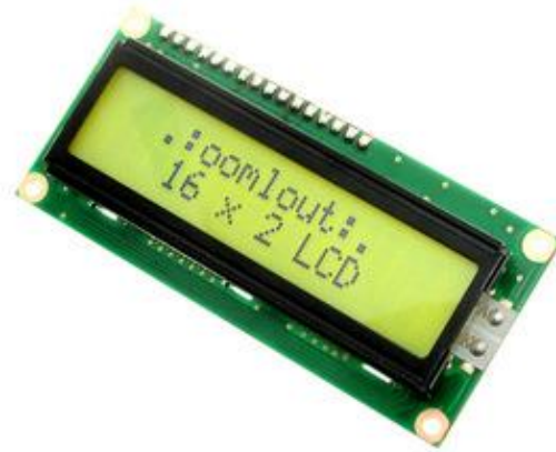
Gambar 2.8 LCD (liquid cristal display) 16x2
