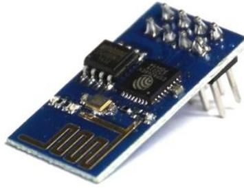
Gambar 2.7 Wireless Module ESP8266
