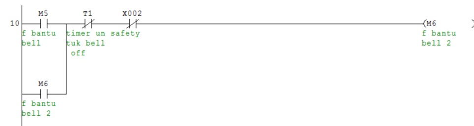
Gambar 4. 40 Ladder Diagram Flag Trigger M5 (flag bantu bell)
