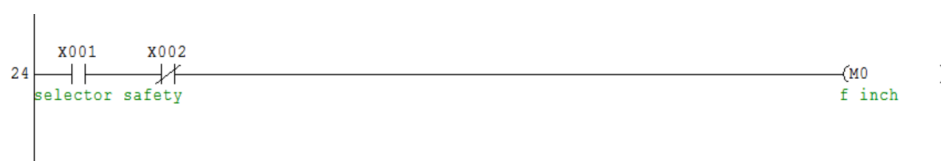
Gambar 4. 26 Ladder Diagram Selector Inching
