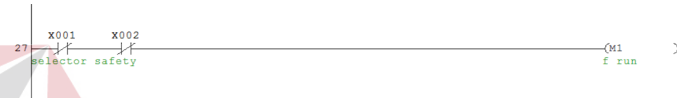
Gambar 4. 38 Ladder Diagram Selector Running
