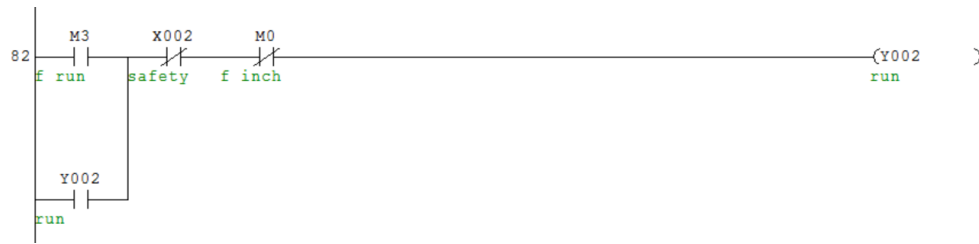
Gambar 4. 45 Ladder Diagram Running
