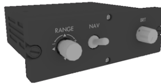
Gambar 2.15 Pilot Display Control Unit
