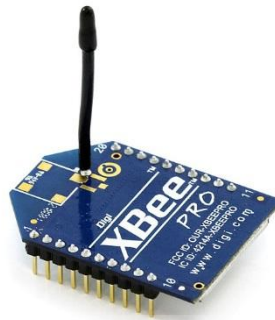
Gambar 2.1. Modul X-Bee Pro. (Digi International Inc, 2009).
