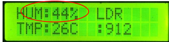
Gambar 4. 5 Nilai Baca Kelembaban Sensor DHT11
