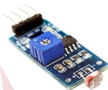
Gambar 2. 6 Sensor Intensitas Cahaya LDR ( Light Dependence Resistor )
