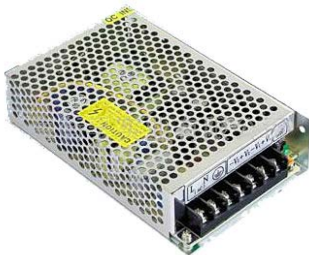
Gambar 2. 15 Power Supply Switching
