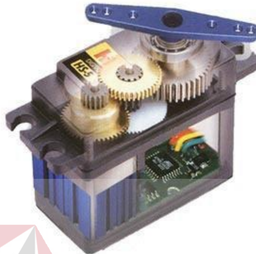
Gambar 2.14. Sistem Mekanik Motor Servo (Widipratama, 2017)
