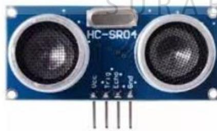
Gambar 2.2 Sensor *Ultrasonic*
