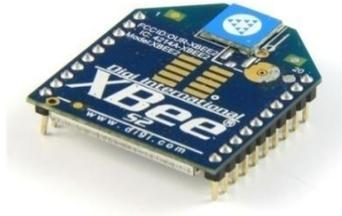
**Gambar 2.7** Xbee Series 2 Chip Antenna
