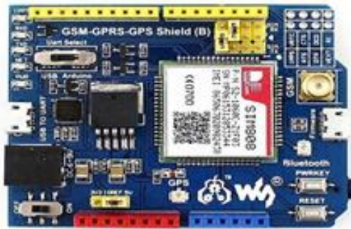
Gambar 2.5 Modul SIM808 GPS/GPRS/GSM Shield
