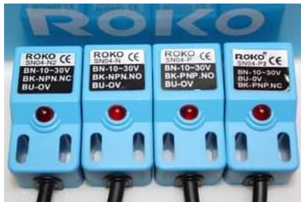
Gambar 2. 15 Sensor Proximity Inductive (Sensor Metal)
