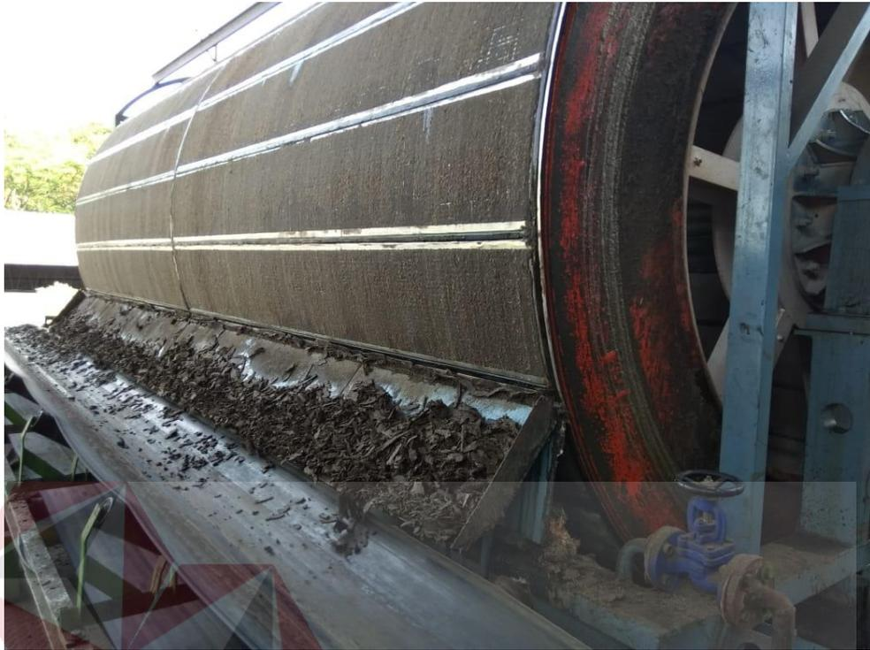
Gambar 4.5 *Rotary Vacuum Filter*
