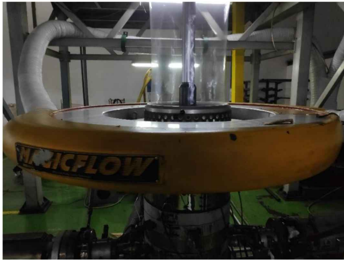
Gambar 4.25 magic flow meniup plastik cair
