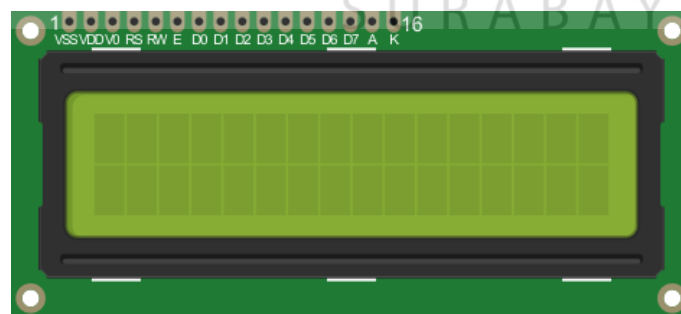
Gambar 2. 12 LCD 16x2 (Liquid Crystal Display)
