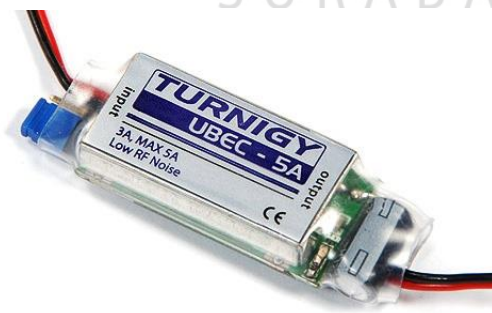
Gambar 2. 13 UBEC – Universal Battery Elimination Circuit
