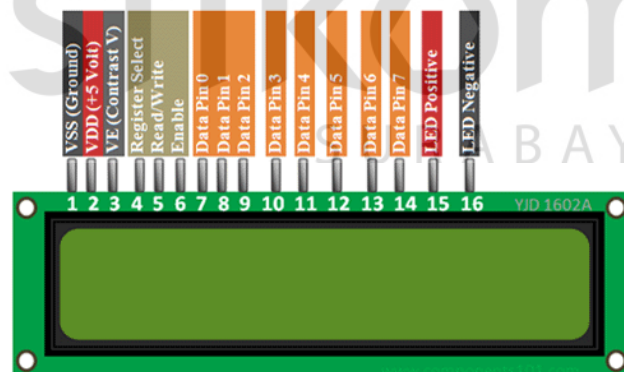
Gambar 3.8 Pin LCD Karakter 16 x 2
