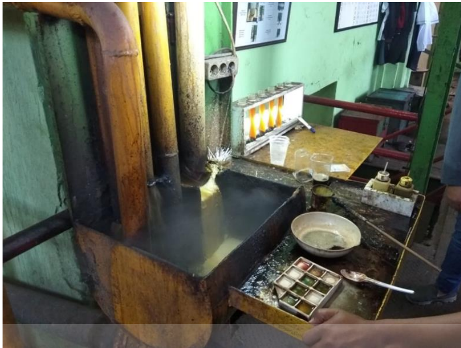
Gambar 3. 5 Proses Sampling pH nira
