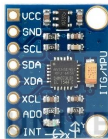
Gambar 2.5. IMU sensor MPU-6050 (Sumber: www.makerlab-electronics.com )
