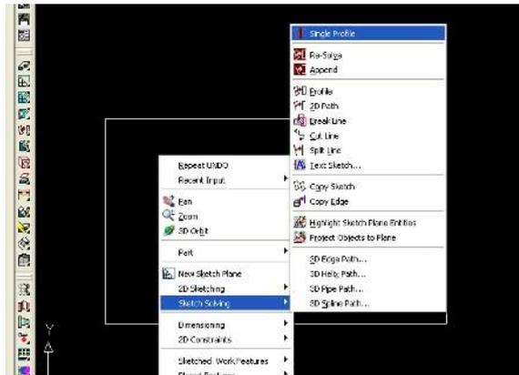
**Gambar 4.17 Menu Profile Mechanical Dekstop**
