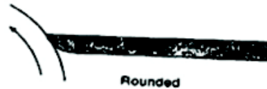
Gambar 3.33 Doctor Blade Tipe Rounded
