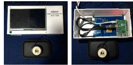
Figure 8. An IoT node for the heart sounds auscultation and identification. Front view of the IoT node on the left side and rear view on the right side
