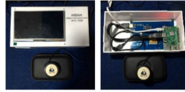
Figure 8. An IoT node for heart sounds auscultation and identification. Front view of the IoT node on the left side and rear view on the right side
