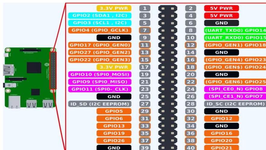
Gambar 2.4 Pinout Raspberry Pi 3 B+ (Sumber : initialboard.com, 2021)
