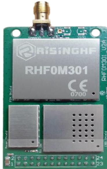
Gambar 2.1 RHF0M301 LoRa Gateway (Sumber : IoTiger.net, 2017)
