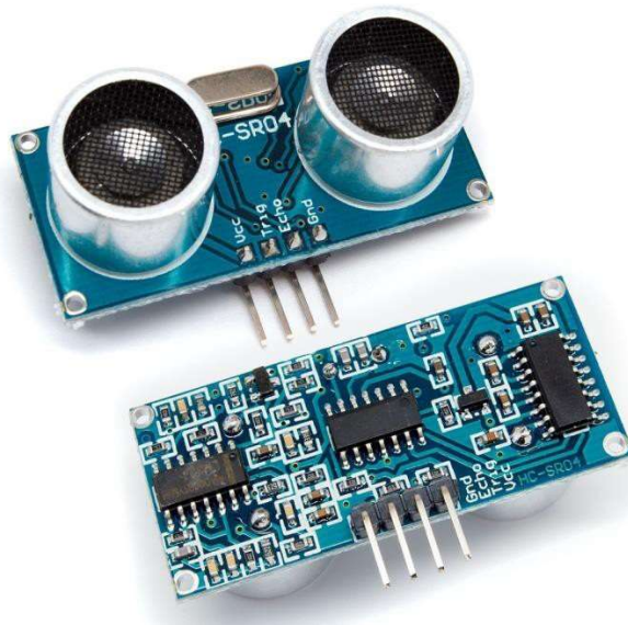
Gambar 2.2 Sensor Ultrasonik HC-SR04 (Sumber: www.shoppe.co.id )
