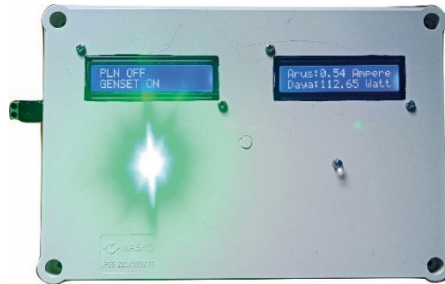
Gambar 4.3 Sensor Tegangan Genset ON
