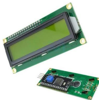
Gambar 2. 6 Lcd 16x2 & I2C (Sumber: www.shopeeindonesia.com )
