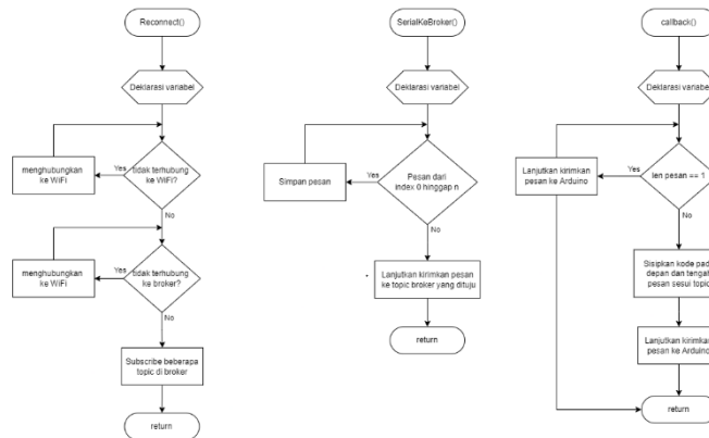
Gambar 3.14 Flowchart fungsi Reconnect(), SerialKeBroker(), dan callback()
