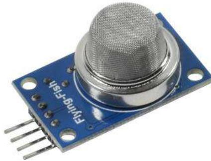
Gambar 2.8 Sensor gas MQ135
