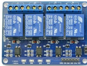
Gambar 2.6 Modul Relay 4 Channel (Sumber : (Component101, 2021))
