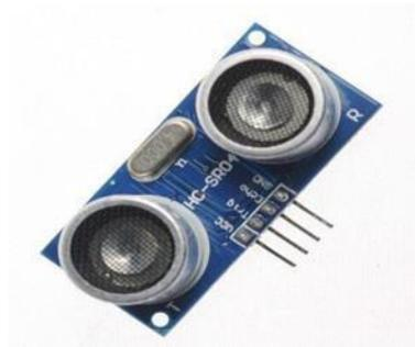
Gambar 2.10 Sensor ultrasonik
