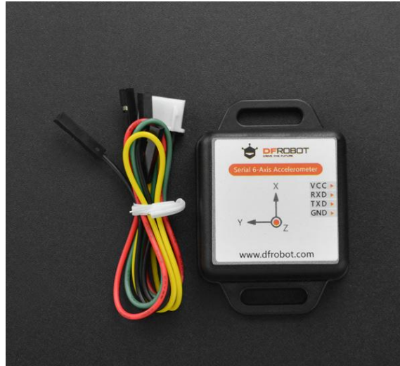
Gambar 2. 5 Dfrobot Serial 6-axis Accelerometer (Sumber: https://www.dfrobot.com/product-2200.html )
