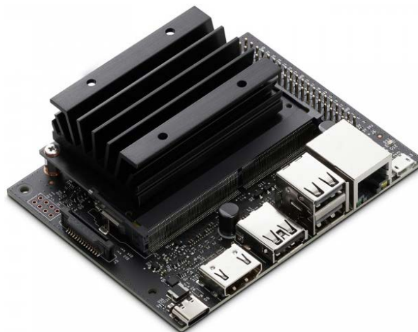
Gambar 2. 1 NVIDIA Jetson Nano (NVIDIA, 2023)
