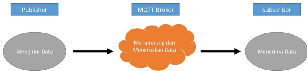
Gambar 3.2 Alur sistem MQTT Broker
