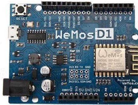
Gambar 2.3 Board WeMos-D1R2 berbasis ESP8266 (Sumber: (ANDY, WEMOS D1 R2 WIFI ARDUINO DEVELOPMENT BOARD, 2019))
