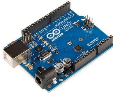
Gambar 2. 9 Arduino UNO (Sumber: https://www.wikipedia.com )
