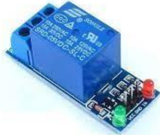
Gambar 2. 3 Relay (Sumber: www.thinkrobotics.com )
