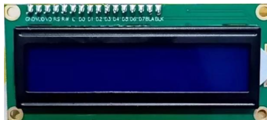
Gambar 2. 11 LCD I2C (Sumber: Bima Prakarsa and Edidas, 2022)
