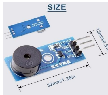
Gambar 3.3 Buzzer Low Level Trigger
